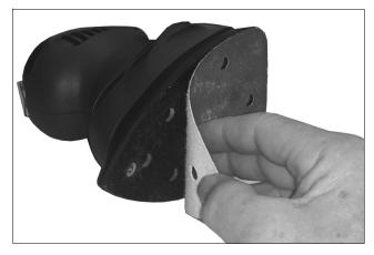
with those in the baseplate (this is necessary for dust extraction). Press the sanding sheet evenly onto the baseplate to attach it.
